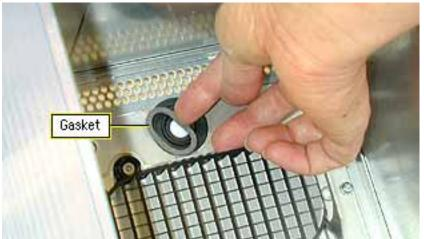
**Caution:** If the power button gasket is not centered correctly in the shell, the computer might not power up. Make sure the power button gasket is level and centered in place.
